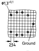
Hole arrangement View in mounting direction
