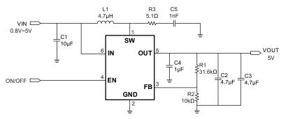
Figure2—V<sub>OUT</sub>=5V Typical Application Circuit
