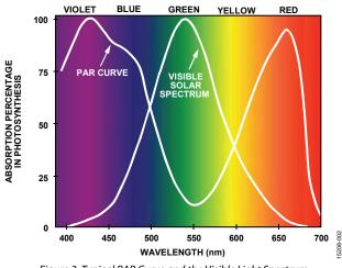
Figure 2. Typical PAR Curve and the Visible Light Spectrum
