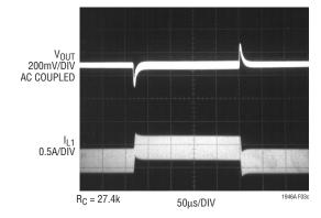
Figure 3c. Transient Response is Well Damped
