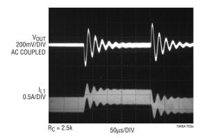
Figure 3a. Transient Response Shows Excessive Ringing
