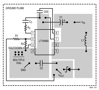
NOTE: DIRECT HIGH CURRENT PATHS USING WIDE PC TRACES. MINIMIZE TRACE AREA AT PIN 1( $V_C$ ) AND PIN 2( $F_B$ ). USE MULTIPLE VIAS TO TIE PIN 4 COPPER TO GROUND PLANE. USE VIAS AT ONE LOCATION ONLY TO AVOID INTRODUCING SWITCHING CURRENTS INTO THE GROUND PLANE
