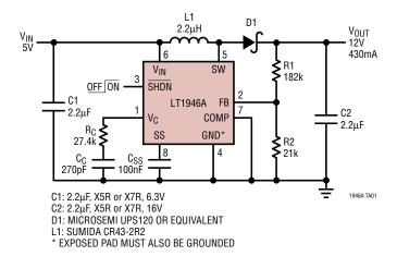
Figure 1. 5V to 12V, 430mA Step-Up DC/DC Converter
