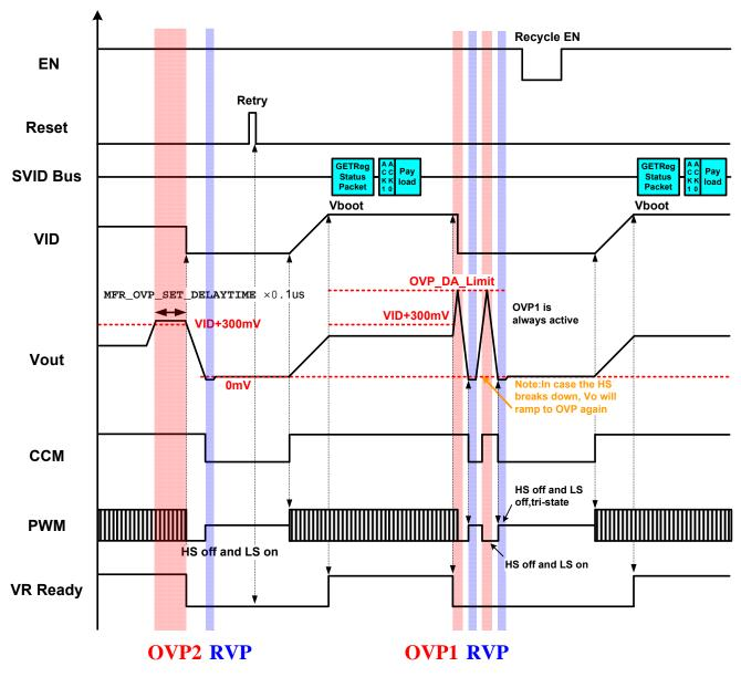
FIGURE 13. OVP and RVP Fault Protection
