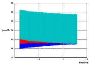
FIGURE 18(b). Phase Current Balance with Σ-Δ Modulation
