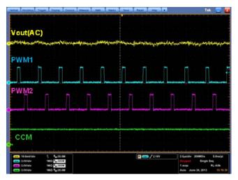
FIGURE 4(a). Steady State with Load @160A
