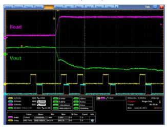
FIGURE 4(b). Load Step Up @ 1kHz
