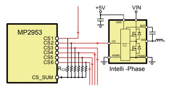
FIGURE 7. Current Sense with Intelli-Phase
