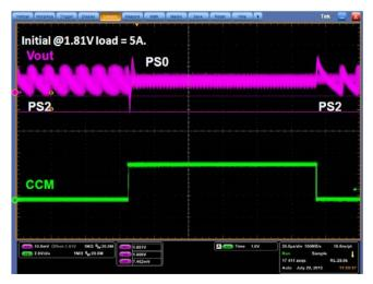
FIGURE 5(b). 1-Phase DCM → 6-Phase →1-Phase DCM
