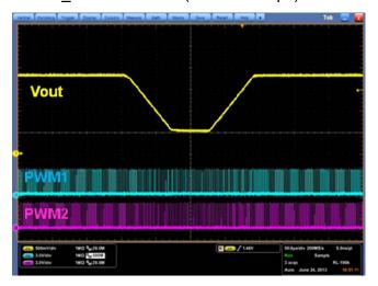
FIGURE 9. SetVID\_Fast Downward → SetVID\_Fast Upward
