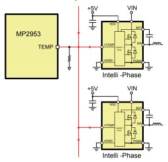
**FIGURE 8. External Temperature Sense**
