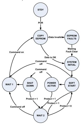
FIGURE 2. System State Machine
