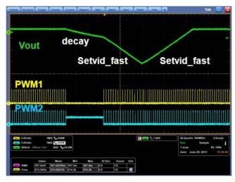
FIGURE 10(a). Decay (Interrupted)→SetVID\_Fast (Interrupted)→SetVID\_Fast (Finished)
