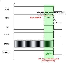
FIGURE 16. Under-Voltage Protection
