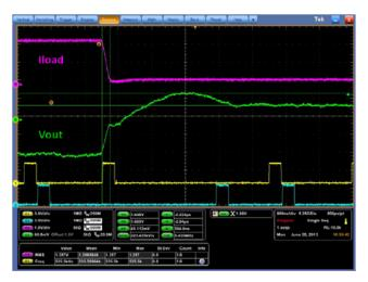
FIGURE 4(c). Load Step Down @ 1kHz
