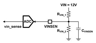
FIGURE 6. VIN Resistor Divider Network
