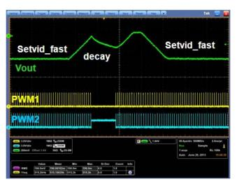
FIGURE 10(b). SetVID\_Fast (Interrupted) → Decay (Interrupted) → SetVID\_Fast (Finished) → SetVID\_Fast (Finished)
