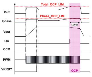
FIGURE 14. OC Protection for Total Current
