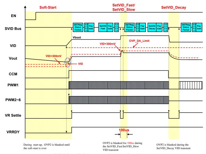
FIGURE 12. OVP Protection Blanking Conditions
