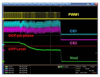
FIGURE17. UVP Triggered when Per-Phase Current is Limited
