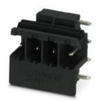
Header, Nominal current: 12 A, Rated voltage (III/2): 320 V, Number of positions: 4, Pitch: 5 mm, Mounting: Soldering, Article with lateral pin exit
