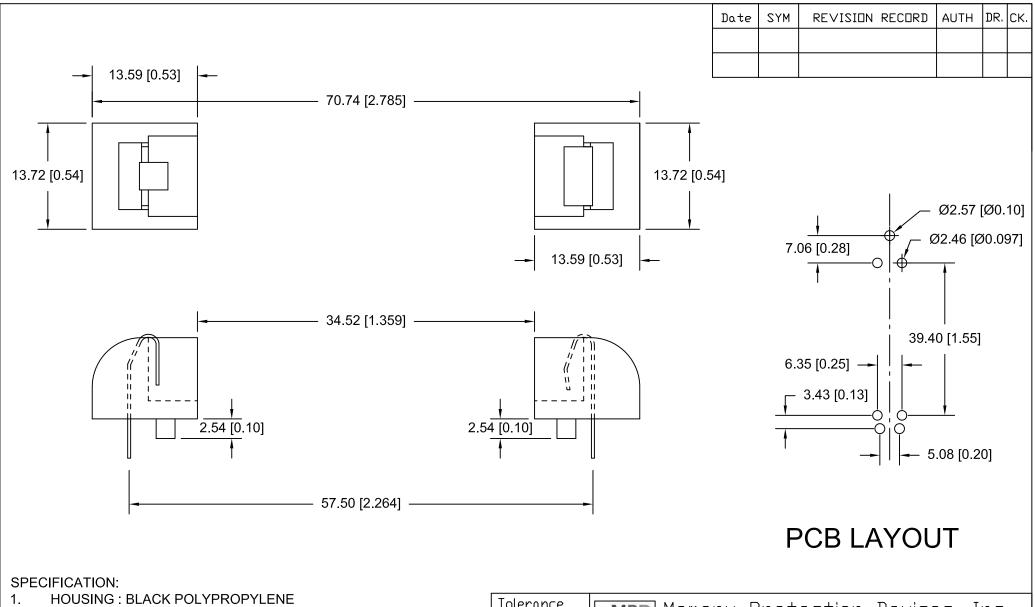
FLAMMABILITY RATING -UL94-HB, UL FILE NO. E216959 TEMPERATURE RANGE: -10°C to +100°C CONTACTS: NICKLE PLATED STAINLESS STEEL ROHS COMPLIANT
