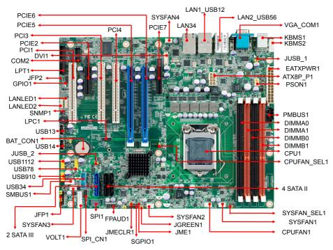
**Board Layout: Jumper and Connector Locations**
