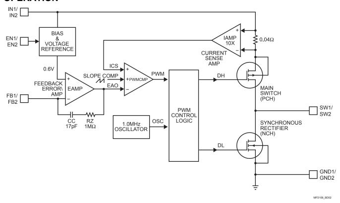
Figure 1—Functional Block Diagram (Diagram represents ½ of the MP2109)
