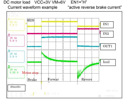
If a direction of rotation is switched while the DC motor is under rotation, torque for reverse rotation is generated. Therefore, the change of rotation takes place more abruptly.
