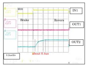
No load VCC=3V VM=12V EN1="H" IN2="L" Time scale expansion "rise time"
