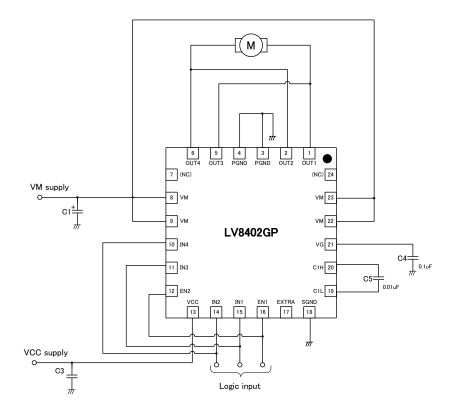
Charge pump circuit is integrated.
