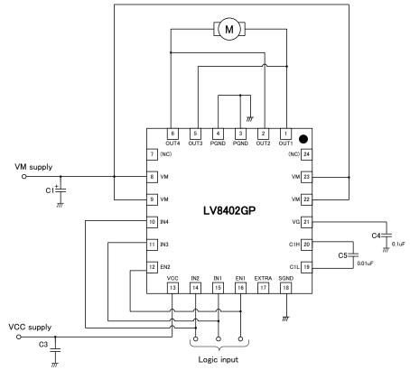
The capacitor C1 and C3 are used to stabilize power supply. And capacitance is variable depends on board layout, capability of motor or power supply.
