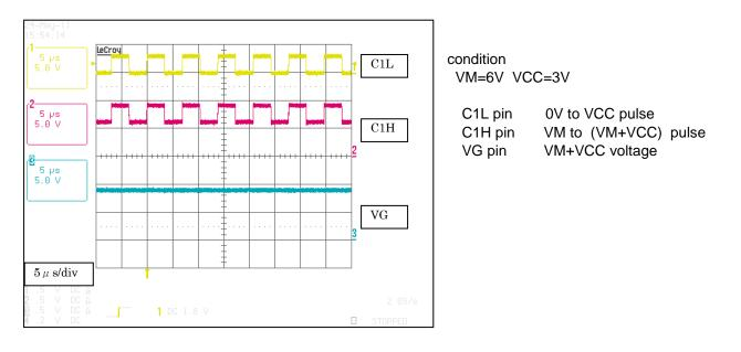
Charge pump waveform example
