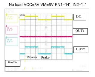
No load VCC=3V VM=6V EN1="H" IN2="L" Time scale expansion "fall time"
