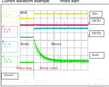
DC motor load VCC=3V VM=6V EN1="H",IN2="L" Current waveform example "motor start"
