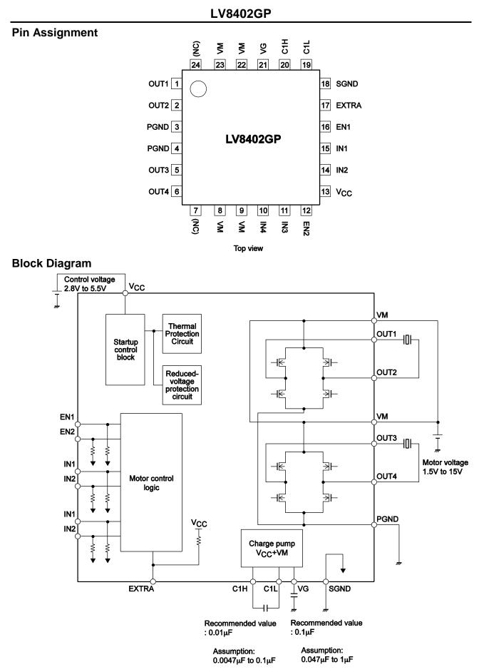
\* Connect a kickback absorption capacitor as near as possible to the IC. Coil kickback may cause increase in VM line voltage, and a voltage exceeding the maximum rating may be applied momentarily to the IC, which results in deterioration or damage of the IC
