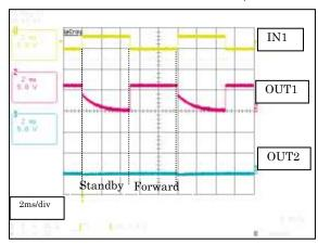
No load VCC=3V VM=6V EN1="H" IN2="L" Time scale expansion "rise time"
