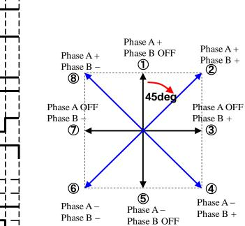
Half-Step Drive (1-2 phase excitation drive) Motor advances 45 degree by inputting 1 step.
