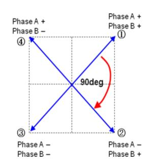
• Full-Step Drive (2 phase excitation drive) EXTRA mode **EXTRA pin = Low** Motor advances 90 degree by inputting 1 step.
