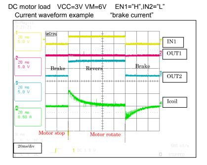
By setting brake mode while the DC motor is under rotation, DC motor becomes short-brake state and thereby decreases rotation count rapidly.
